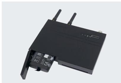
The LED indicators of the PWU provides information about the power status, wired/wireless activation, charging status and battery level.
